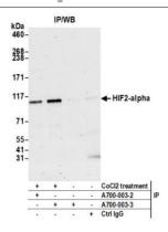
Detection of human HIF2-alpha by western blot. Samples: Whole cell lysate (50 μg) from HepG2 and 786-O cells treated with 200 μM CoCl2 (+) or mock treated (-). Antibody: Rabbit anti-HIF2-alpha recombinant monoclonal antibody [BL-95-1A2] (A700-003-T lot 3) used at 1:1000. Secondary: HRP-conjugated goat anti-rabbit IgG (A120-101P). Chemiluminescence with an exposure time of 75 seconds.
