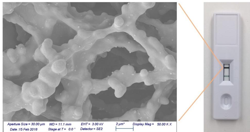
**Figure 2:** Gold nanoshells bound to a nitrocellulose membrane..
