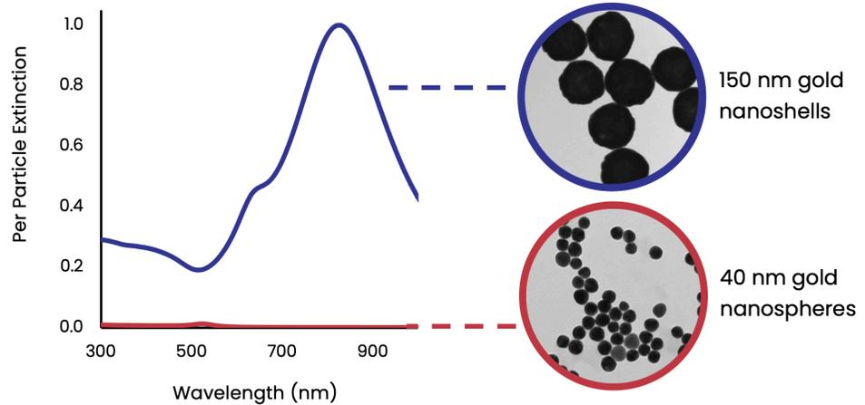
**Figure 1:** Extinction per particle of traditional 40 nm gold nanospheres versus 150 nm gold nanoshells.
