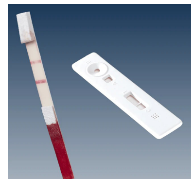
Figure 13: Lateral flow assay with sample pad that has a red blood cell filter. Image from mdimembrane.com
