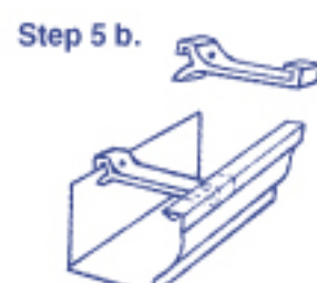
Hidden Hanger Insert hanger underneath front lip and over back of trough and screw into fascia board.
