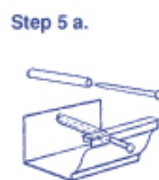
Spike and Ferrule Insert ferrule into gutter and drive spike through gutter, ferrule and fascia board.
