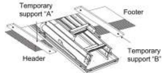
**NOTE:** With the attic ladder positioned on the temporary support boards, be sure the plastic bushings are present and have not moved or fallen out before proceeding.
