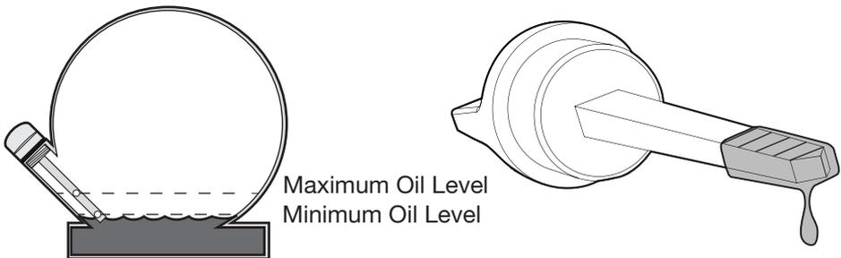
4. Reinsert the dipstick and tighten securely.
