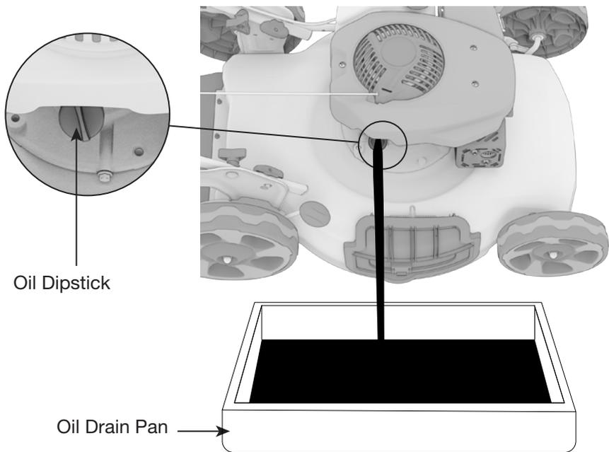
1. Tilt the lawn mower towards the oil drain pan, have a container ready to catch the oil and remove the dipstick.
