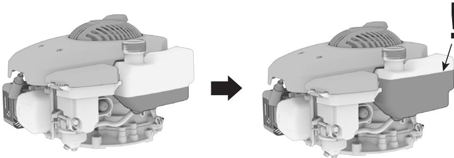
3. Tighten the fuel cap securely after refilling.
