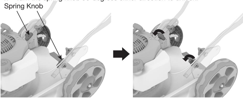
2. Choose a higher or lower bracket hole to set your handle height preference. Then turn the spring knob back 90-degrees until the silver bolt goes through that bracket hole.
