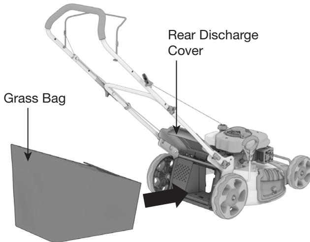
1. Clip the plastic clips of the grass bag over the metal frame and make sure they are fully secured to the metal frame.
