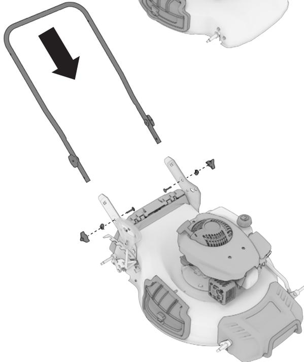
2. On each side of the upper handle, insert the bolt and secure with saddle washer and handle knob.
