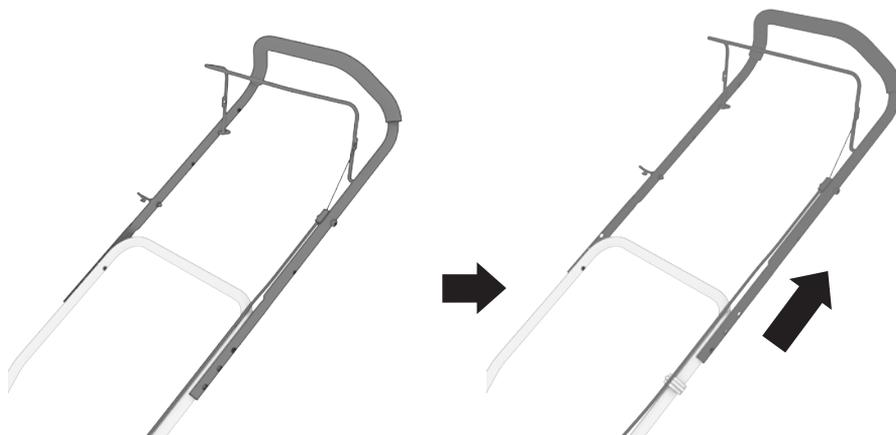
3. Fix it to lower handle by using the hand knobs and the bolts on each side.
