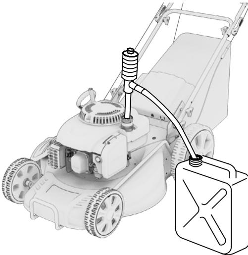
1. Turn OFF the engine. Remove the fuel cap.
