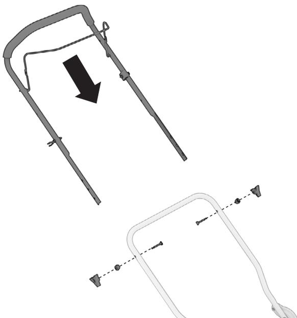
3. Ensure power lever cable is resting above lower and upper handles as pictured.
