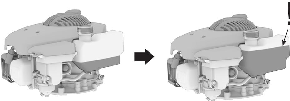
3. Tighten the fuel cap securely.
