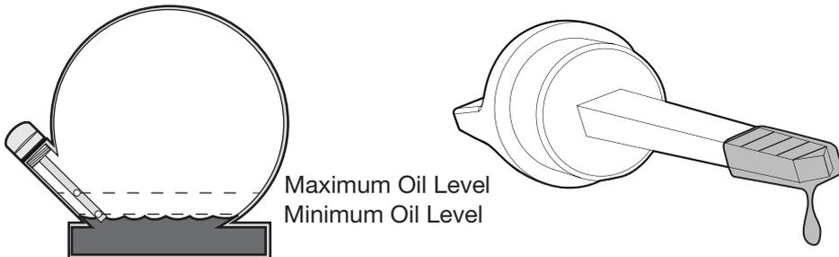
4. Reinsert the dipstick and tighten securely.
