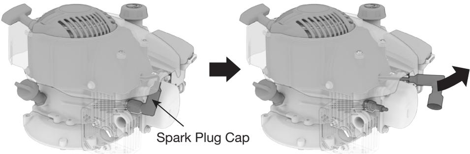
3. Remove the spark plug, dry it, and then reinstall it.
