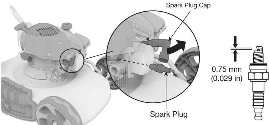
1. Remove the spark plug cap.
