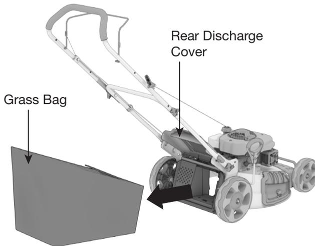
1. Use one hand to lift up rear discharge cover and the other to take off the grass bag. The rear discharge cover automatically falls down after removing the grass bag and closes the rear chute opening.
