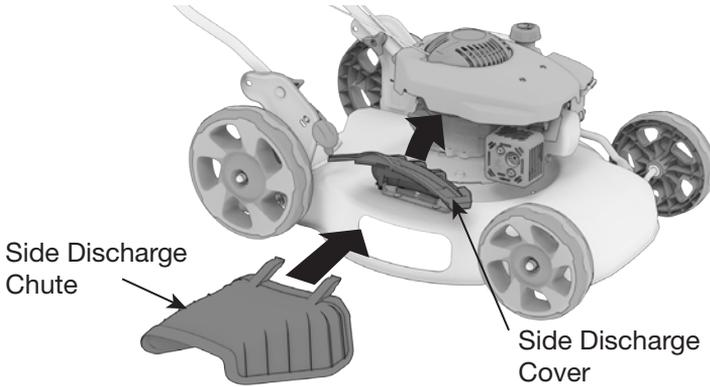
2. Release the side discharge cover to secure the chute in position.
