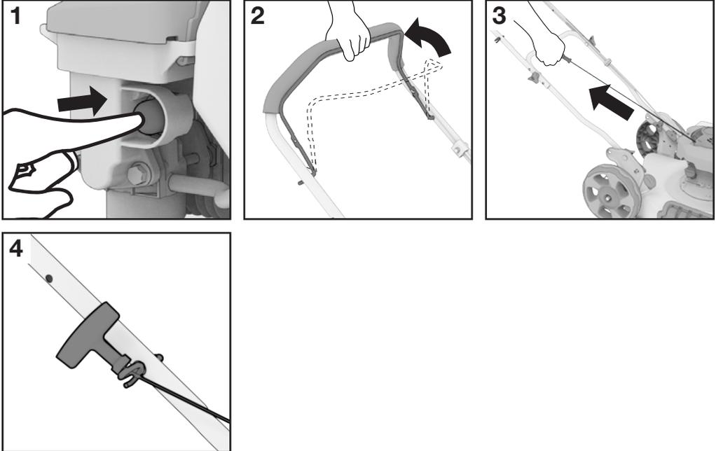
1. In cold weather ONLY, push the primer bulb 1-2 times.
