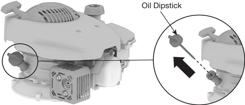
3. Check the oil level by reinserting the oil dipstick *without* screwing it back in. Remove the dipstick and examine the oil level. If the level is at or below the minimum oil level marked on the dipstick, refill to the maximum oil level mark.
