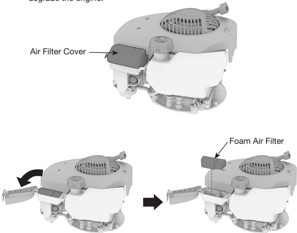
1. Loosen the nut and remove the air filter cover. Remove the air filter housing and elements and inspect for cleanliness.
