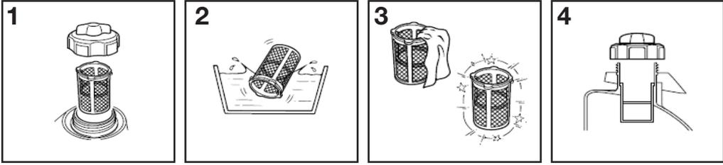
1. Remove the fuel cap and filter.
