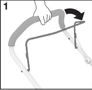
1. Release the power lever. It will return to its initial position and the engine will automatically switch off.
