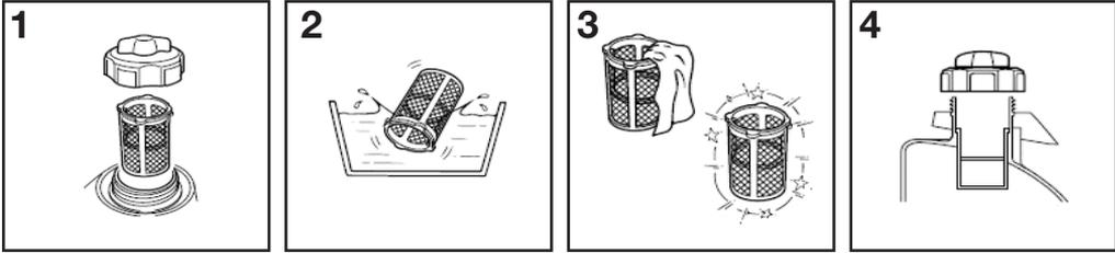
1. Remove the fuel cap and filter.
