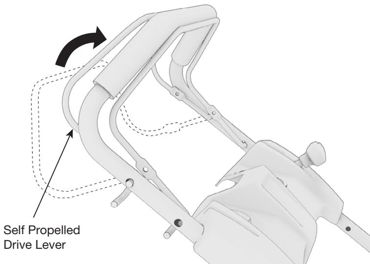
To stop moving the lawn mower, just simply release the self propelled drive lever.
