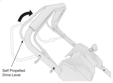
To stop moving the lawn mower, just simply release the self propelled drive lever.
