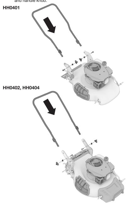
**2.** On each side of the upper handle, insert the bolt and secure with saddle washer and handle knob.
