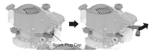
3. Remove the spark plug, dry it, and then reinstall it.
