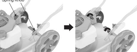
2. Choose a higher or lower bracket hole to set your handle height preference. Then turn the spring knob back 90-degrees until the silver bolt goes through that bracket hole.
