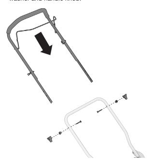
**3.** Ensure power lever cable is resting above lower and upper handles as pictured.
