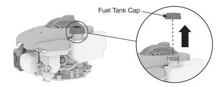
2. Add fuel carefully. DO NOT fill into the base of the fuel neck.
