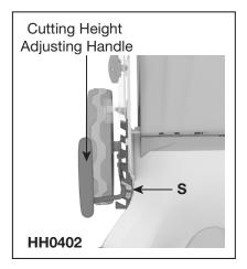
**3.** Release handle from upright position, fold down. Lock into vertical storage position.
