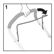
**1.** Release the power lever. It will return to its initial position and the engine will automatically switch off.
