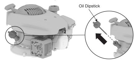
Check the oil level by reinserting the oil dipstick without screwing it back in.
