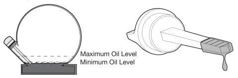
4. Reinsert the dipstick and tighten securely.
