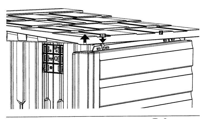
Ensure Front Roof (J) is positioned against the back wall tongues.
