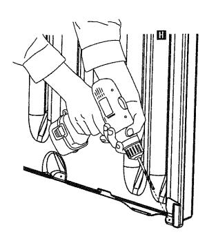
Snap Front Right Side (H) into Front Floor (A). Hold Front Right Side (H) upright to prevent it from falling (until Right Back (F) is installed).
