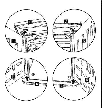
**Prom** inside the shed, install four **Screws (AA)** into the roof, two on each side wall.
