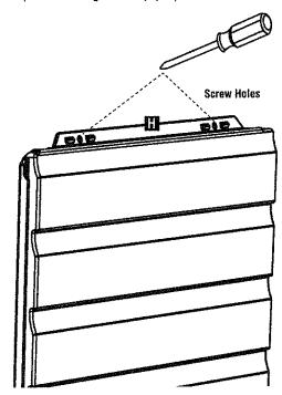
Drill a pilot hole (using 1/8" drill bit) in front lower corner at location indicated by screw target.
