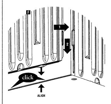
Install Wall Connector (Q) 5 places, connecting Left Back and Right Back Panels (D and F).
