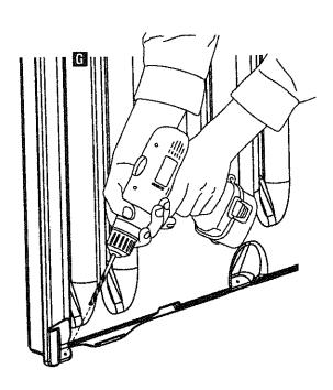
Snap Front Left Side (G) into Front Floor (A). Hold Front Left Side (G) upright to prevent it from falling (until Left Back (D) is installed).
