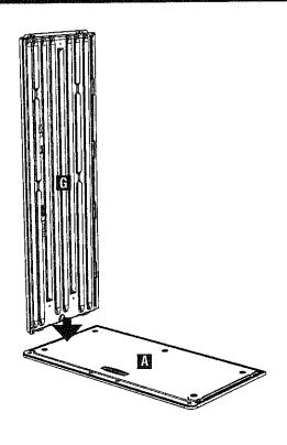
**a.** Using a screwdriver, punch out the screw holes on the top of **Front Left Side (G)** 2 places.
