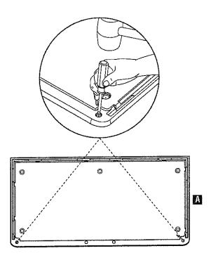
**D**. Drill pilot hole through top surface of floor, 2 places on **Front Floor (A)**.
