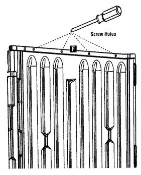
Connect Right Back (F) onto dovetails of Front Right Side (H).
