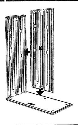
Using a screwdriver, punch out the screw holes on the top of Left Back (D) 4 places.
