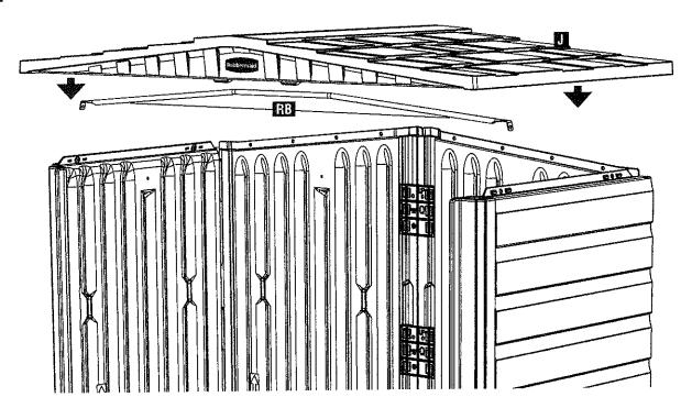
Slightly raise front edge of roof enough to allow positioning of **Roof Brace (RB)** onto the side walls as shown. Lower the roof onto the walls and align **Roof Brace (RB)** into pocket in **Front Roof (J)**.
