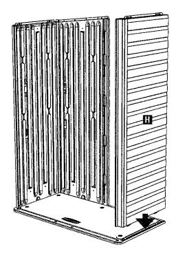
Using a screwdriver, punch out the screw holes on the top of **Front Right Side (H)** 2 places.
