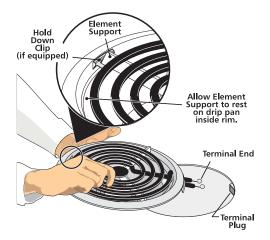
Figure 28: Removing surface elements and drip bowls
