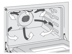
Figure 19: Air movement using convection
