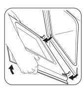
Figure 32: Holding door for removal
