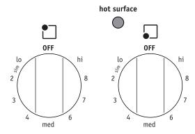
Figure 5: Hot surface indicator light location
