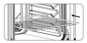
Figure 9: Removing, replacing, and arranging racks
