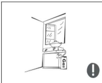
In the event of a gas leak, please turn off the gas valve and then open the doors and windows. Do not unplug the freezer or any other electrical appliances as that may create a spark and cause a fire.
