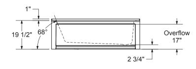
Wood support design may vary. Single Integrated tiling flange: 1" height x 1/4" thickness (shown)
