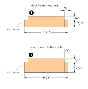
The door width should be  $12^{3/4}$ " wide. Test fit the rail tenons into the side frames to ensure this door width.
