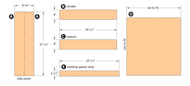
In the side panel, cut a  ${}^{3}/{}^{4}$  x  ${}^{1}/{}^{4}$  deep groove to accept the top piece and a  ${}^{3}/{}^{4}$  x  ${}^{1}/{}^{4}$  deep rabbet to accept the bottom piece.
