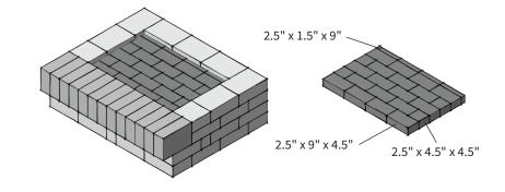
**NOTE:** Do not put silicone on any of the fire brick. They should only be dry stacked, allowing for any bricks to be replaced if necessary. Fill any gaps between the Quarry Stone with silicone. Fill these gaps from the interior of the fireplace so no silicone is shown from the outside.
