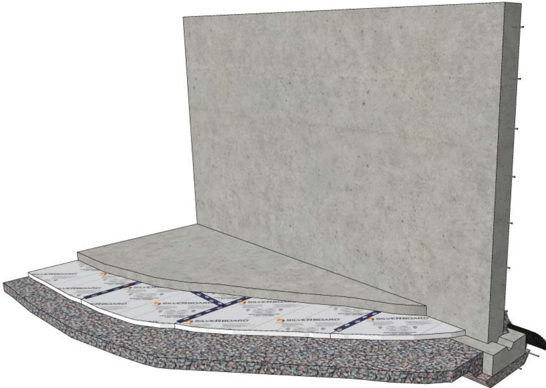
Application of SilveRboard UC below concrete slab
