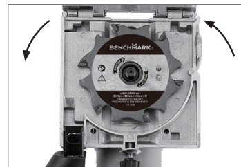
Fig. 23. Blade installed with teeth correct direction.
