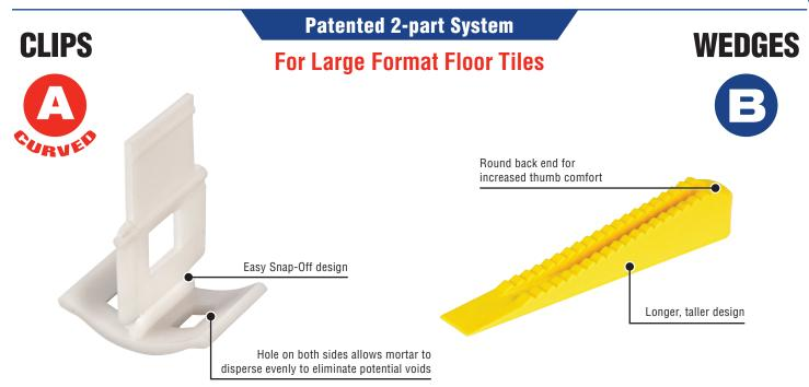
Designed for quick installation, the LASH® Tile Leveling System (sold separately) reduces costly call backs by ensuring that the finished floor surface is lippage-free. It is the perfect system to use with large-format rectified porcelain, thin porcelain tile, marble and stone where narrow grout joints are required, or with tiles of different thickness. This fast, simple system is the most cost effective installation method on the market to eliminate lippage.
