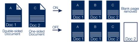
When scanning a batch of documents the ADS-2000 will detect and remove any blank pages to save time and space while archiving.
