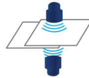
To prevent more than one document being scanned at one time the ADS-2000 uses ultrasonic multi-feed detection that ensures no documents are missed.
