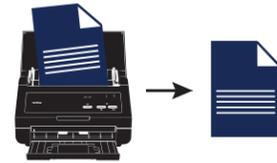
To ensure that all your documents are scanned as they should be the ADS-2000 automatically corrects any skewed documents that are fed into the machine.
