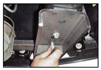
**8.** Start factory bolts in the front holes of base plate.
