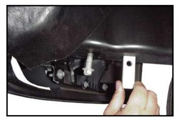
Reinstall factory bolt into rear tow hook hole in frame, also Insert nut strip into rear hole and center over hole.
