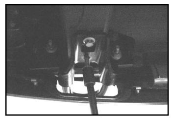
5. Remove tow hooks, on each side, by removing front bolt and loosening rear bolt from each hook. Leave approximately 1-1/8" of threads showing. This will aid in the installation of base plate. The tow hooks will not be reused.
