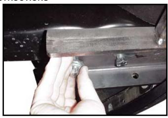
With an assistant put base plate up from rear and slide bolt through keyhole. Insert the other bolts with lock and flat washers and snug. Remove center bolts, add lock and flat washers. NOTE: Use Blue LOCTITE. on all bolts and torque bolts according to the chart on front page.
