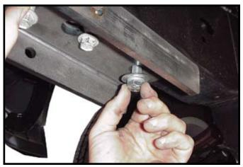
9. Insert supplied 1/2" x 2" Gr. 5 Hex Head bolts, 1/2" Lock washers, and 1/2" thick washers in rear holes (one on each side) and tighten all bolts. NOTE: Use Blue L@CTITE\* on all bolts and torque bolts according to the chart on front page.
