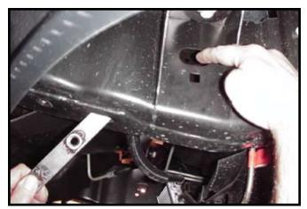
3. For 2wd insert nut strip into frame (NOTE: Long tab end must go to front to vehicle). Line up nut strip with holes in frame and start center bolt without washers. Leave approximately 1-1/8" of threads showing. This will aid in the installation of base plate.
