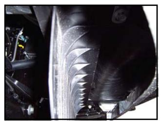
1. If equipped with an air dam remove and discard or relocate the air dam, bolts, and nut clips
