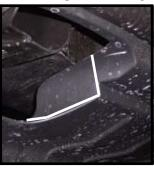
2a. Four wheel drive proceed to step 4. With out tow hooks cut facia according to picture shown above. For all 2009 & newer 4wd model trim as shown on right. NOTE: For vehicles with tow hooks skip to step 5.
