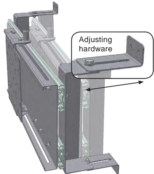
**STEP 3 Secure the television to mounting plate:** Line up the hole pattern on your television with the matching hole pattern on the universal mounting plate as close to the center as possible. Using the appropriate mounting hardware, washers, and optional spacers, secure the television to the mounting plate. This can be done without removing the mounting plate, figures are shown without bracket for illustration purposes only.
