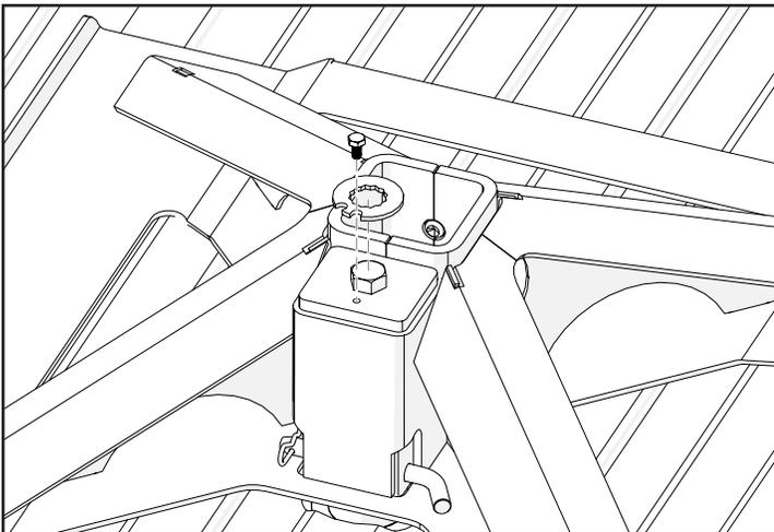
3. When coupler pin is installed, tighten top coupler bolt to 30 ft/lbs. Install bolt retainer over bolt and secure retainer with the 1/4" bolt.
