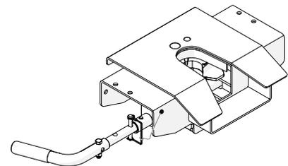
To uncouple, remove safety pin, pull handle straight out until the jaw locks open. If jaw will not stay open, install safety pin in second handle hole just outside of frame handle bushing.
