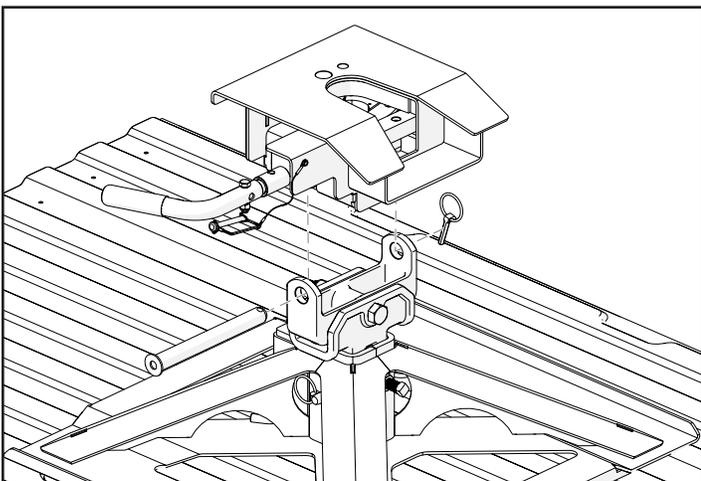
5. Install 5th wheel head with the 1" pin.
