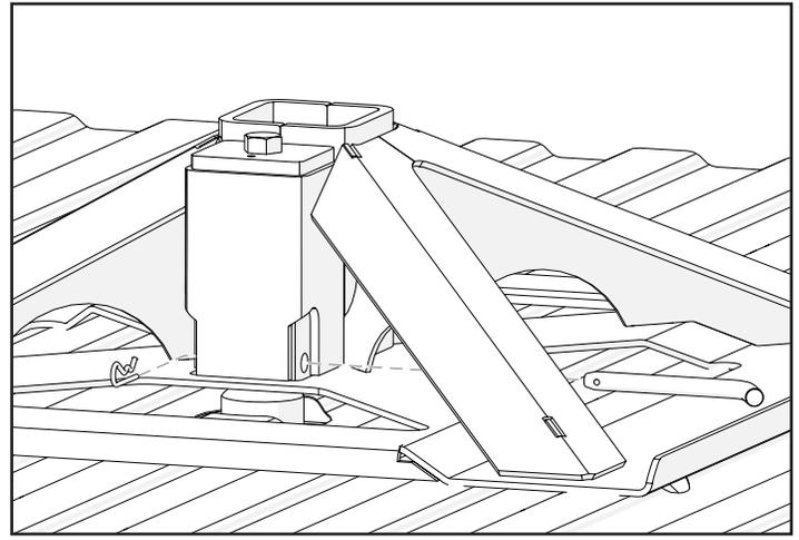
2. Slide coupler pin into coupler hole, making sure pin goes under gooseneck ball. Top coupler bolt may need to be loosened for pin to go under the ball.
