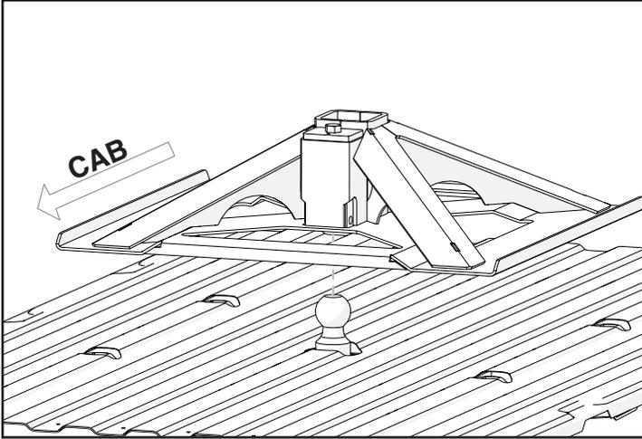
1. Place Recon base over gooseneck 2-5/16" ball so ball fits into the recon ball coupler. NOTE: Ball coupler socket goes towards cab of truck.
