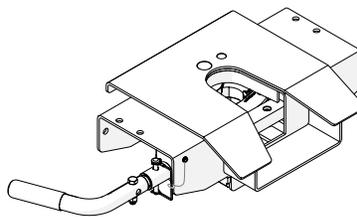
With handle in "Ready to Couple" position, back-up tow vehicle to couple trailer and hitch. Insert safety pin thru tab and hole in handle. NOTE: Ensure safety lock pin is inserted properly. Apply trailer brakes before jacks are raised and wheel chocks are removed.
