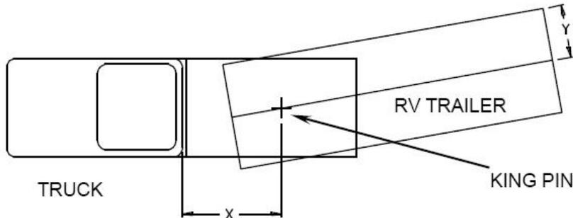
Rule of thumb: The distance from the back of the truck cab to the center of the rear truck axle ("X"), should be approximately 4 inches greater than one-half the trailer width ("Y")
