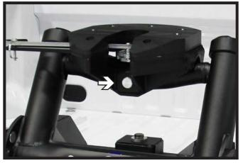
Insert the pin through the front of the hitch and then insert the clip on the back of the hitch to secure the hitch head to the shock towers.
