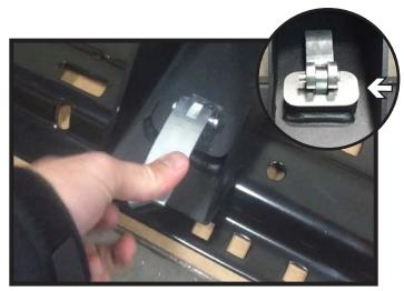
4. Close cam tabs to attach the hitch base to the rails.
