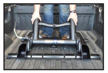
Move the shock towers towards the cab of the truck and manually reengage the locking handle.
