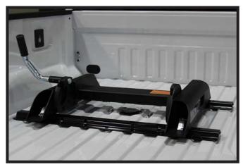
3. Set the hitch base onto the industry standard rails (ISR).
