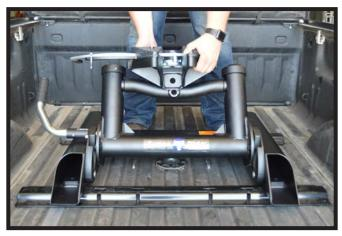
Set the hitch head on top of the shock towers.
