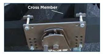
If your trailer tongue frame has a cross member or other equipment that prevents attachment of the clamp-on latches you will want to use the Bolt-On Latches (BXW4021).
