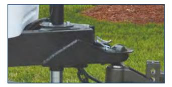
If your trailer has a coupler welded underneath the frame you will need to replace the hitch head with the Underslung Hitch Head (BXW4012)
