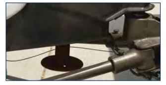
The Swaypro hitch comes with a Standard Hitch Head (BXW4011) fitting a Standard Coupler welded to the top of the trailer frame.
