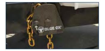
The Swaypro hitch comes standard with Clamp-On Latches (BXW4010). Designed for trailer tongue frames without cross members or equipment blocking attachment of the latches.
