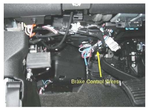
Connect the brake control to these wires as follows.
