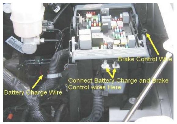
The battery charge wire and the brake control wire have different size eyelets on them and will connect to the threaded studs under the Gray handle of the front of the fuse box. The two studs are also different size.
