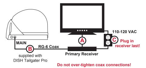
When you plug in the receiver (make sure outlet is powered), the green power light on the front of the receiver should illuminate or begin cycling on and off.
