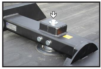
4. Using a torque wrench tighten the top bolt on the hitch base to 45 ft./lbs. to secure the base into place. Ensure that the base is solid to the truck bed. Then tighten the two (2) 5/8" bolts on the front side of the hitch, nearest to the cab, to eliminate any play around the ball housing.
