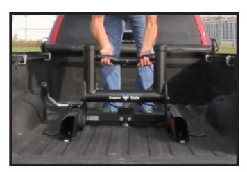
Center the shock towers over the hitch base vertically. Align the two (2) pins, one (1) on each side, with the grooves on each side of the hitch base and set into place.
