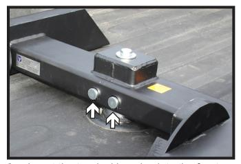
Insert the two locking pins into the front of hitch base and attach the clips. (Some gooseneck hitch balls may sit too low for proper hook up of the BXR6200. A "high rise" gooseneck ball may be required).
