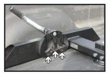
2. Recommended clearance between truck bed and 5th wheel trailer is 6-8 inches. To adjust the height of the Super Ride's hitch head remove the three (3) bolts holding the roll guide plate and adjust appropriately. Do this for both driver side and passenger side ensuring that both sides are equal in height.
