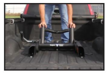
4. Move the shock towers towards the cab of the truck and manually reengage the locking handle. Reinsert quick release pin into the roll guide plate.
