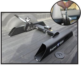
Remove the quick release pin from the roll guide plate (inset). Then release locking handle by pulling the handle towards the rear of the truck bed. Then pull the handle outwards and then towards the truck bed again.
