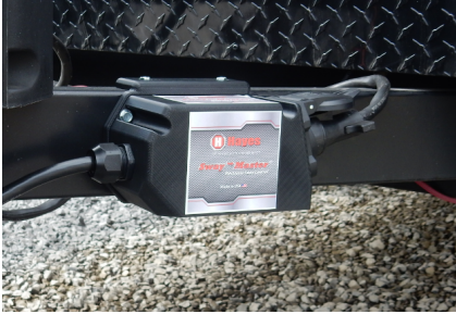
Fig. 1- Correct mounting position shown. Top of Sway Master™ must have an unobstructed view of sky.
