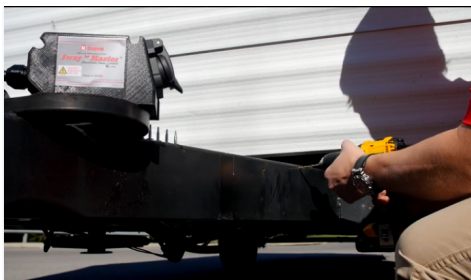
Fig. 3- Drill holes in trailer tongue
