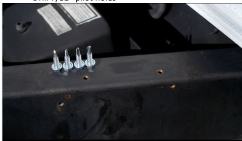
Fig. 4 – Pilot holes shown with included self-tapping screws.
