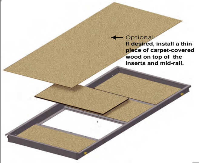
Figure 2: Install carpet-covered wood panels into inner rail assembly.
