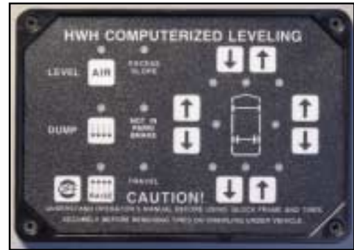
The HWH Air Leveling System features computer (touch panel) control and our HWH Levelize Indicator Light System. The control pad can be dash mounted for operator convenience.
